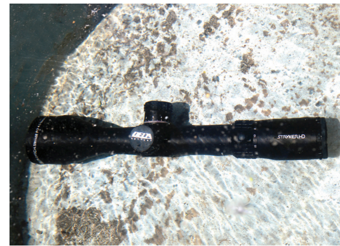
The Stryker in a bucket of grey water for its submersion test.
